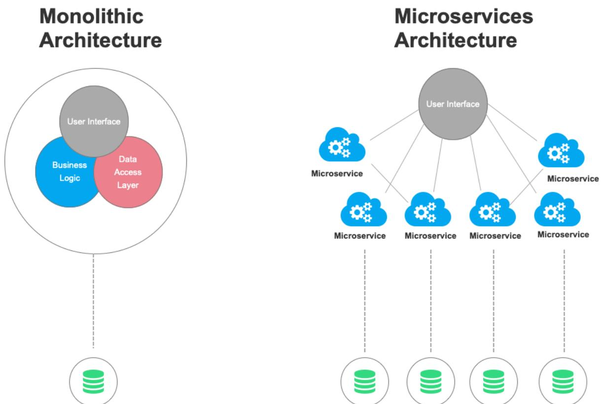
**Figure 7: Monolithic vs. Microservices architecture conceptualization**
