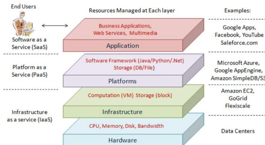
**Figure 8: Typical Architecture for Cloud Computing Environments**
